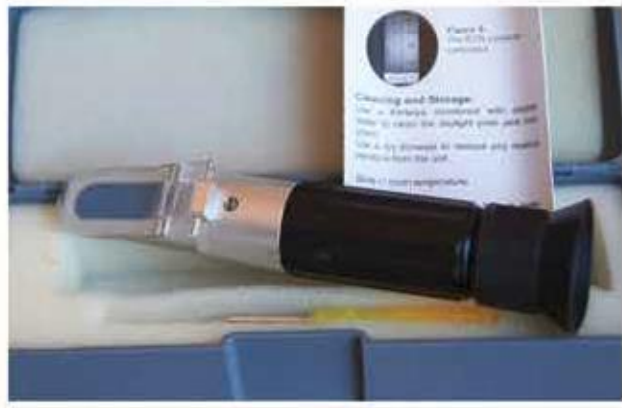
A colostrum refractometer is a portable instrument for analyzing mare colostrum quality. Only a few drops of colostrum are required and the entire test can be completed in less than a minute.
